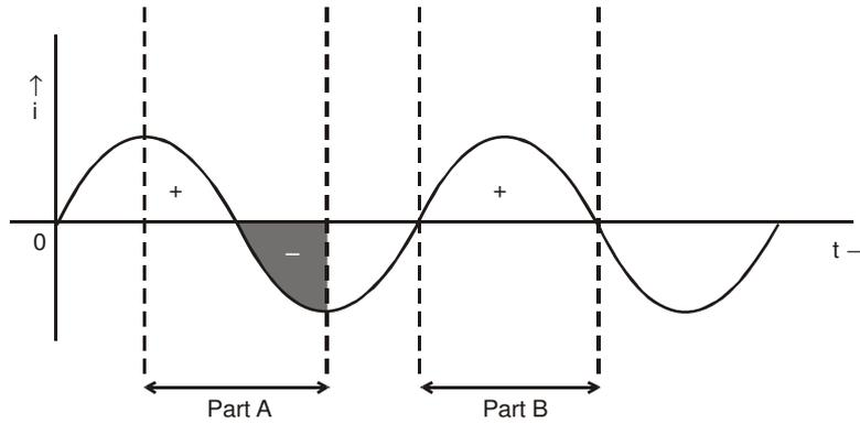
Figure shows two parts A and B, each half cycle. In part A we can see that the net area is zero
