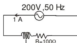
For the bulb to be operated at its rated value the rms current through it should be 1A
