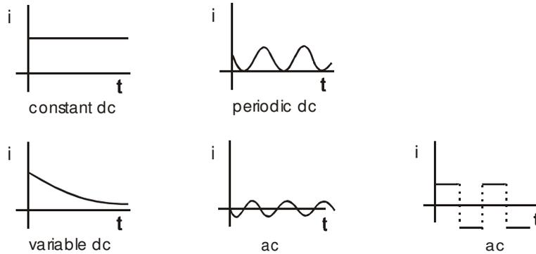
If a function suppose current, varies with time as  $i = I_m \sin(\omega t + \phi)$ , it is called sinusoidally varying function. Here  $I_m$  is the peak current or maximum current and  $i$  is the instantaneous current. The factor  $(\omega t + \phi)$  is called phase.  $\omega$  is called the angular frequency, its unit rad/s. Also  $\omega = 2\pi f$  where  $f$  is called the frequency, its unit  $s^{-1}$  or Hz. Also frequency  $f = 1/T$  where  $T$  is called the time period.
