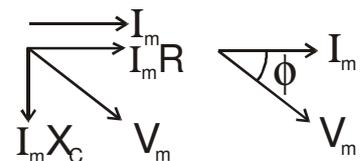
**Ques.** An AC source producing emf  $\xi = \xi_0 [\cos(100 \pi \text{ s}^{-1})t + \cos(500 \pi \text{ s}^{-1})t]$  is connected in series with a capacitor and a resistor. The steady-state current in the circuit is found to
