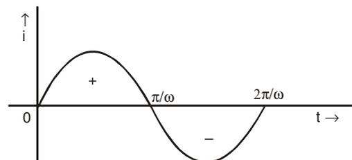
It can be seen graphically that the area of  $i-t$  graph of one cycle is zero.
