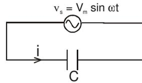
$X_C = \frac{1}{\omega C}$  and is called capacitive reactance. Its unit is ohm  $\Omega$ .
